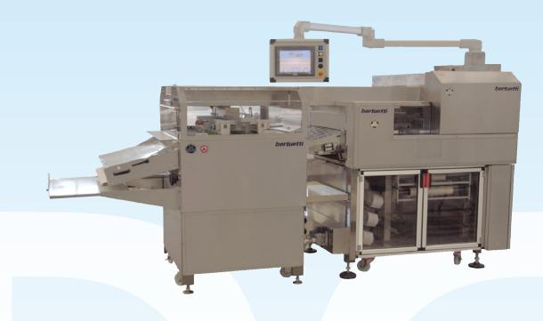
The unique Bertuetti SVG3 combines a stress free dough divider with a gentle rounding system to become the complete machine for the modern bakery. Variable speed makes it suitable for all production requirements and it is suitable for all dough types, from direct dough's through to very hydrated, long rested/fermented dough's. In short, it is the most dynamic dough processing machine on the market today. It is the machine for today and tomorrow.
